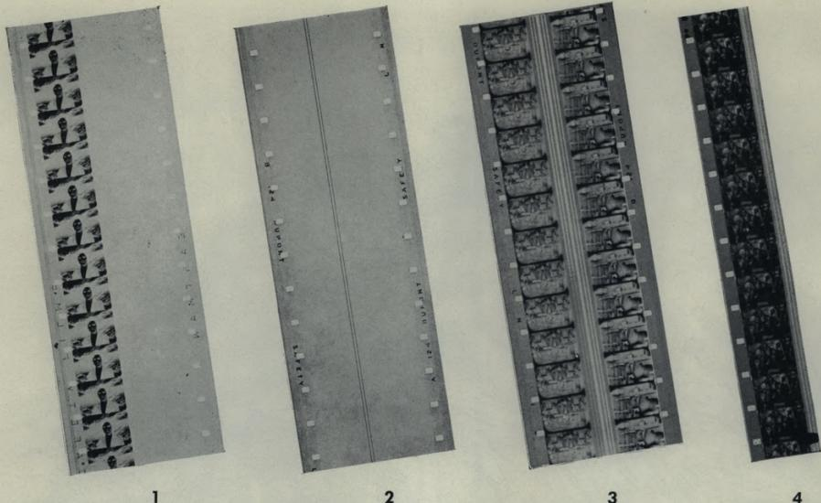
EVOLUTION OF A 16mm black-and-white and sound print made by the 35/32mm printing method. The first film is the 35/32mm picture dupe negative; 2 is 35/32mm sound negative; and 3, 35/32mm double composite print. Strip No. 4 is the completed 16mm print after being
